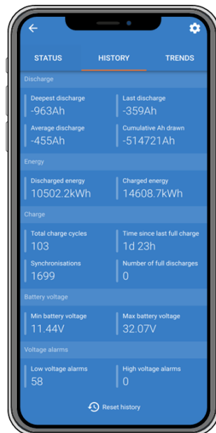
The VictronConnect app battery monitor history screen.
