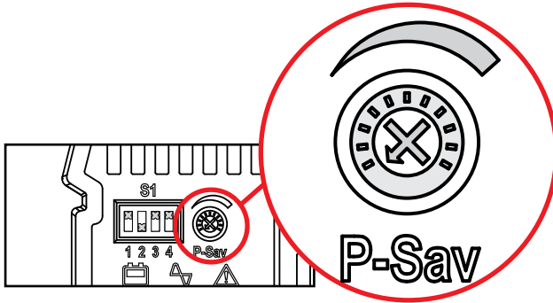
FIGURE 2.1.4.1: Power Saving Load Adjustment
