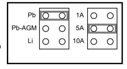
In order to set the charging parameters, remove both jumpers and use the USB interface on page 10.
